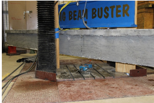
Figure D.1b Uncracked Under Load
