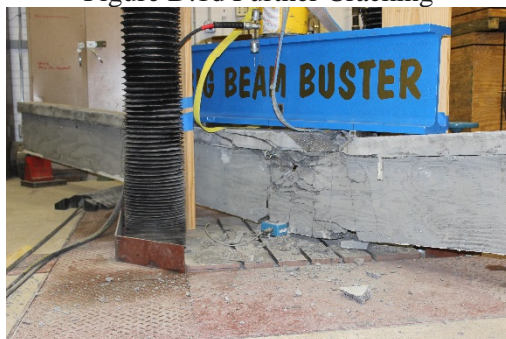
Figure D.1f Ultimate Failure
