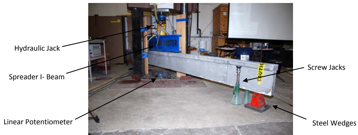
Figure 5: Four Point Bending Test Set Up
