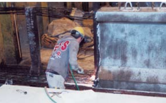
For this bridge girder being manufactured, cutting torches are being used to detension the strand.
